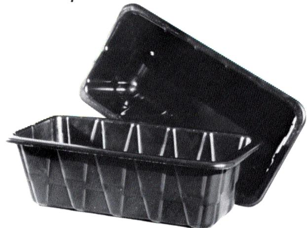
The use of a plug will add to the initial tooling costs. These costs are often quickly regained in subsequent material savings. Plugging procedures provide a substantial improvement in wall uniformity and permit the use of lighter gauge sheet to form equivalent parts. To illustrate potential improvement, the flower box shown in Figure 7 was formed by both female drape and plug-assist techniques in the same mold.
